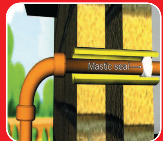
Fig. 11 Pipe Through Wall Detail
